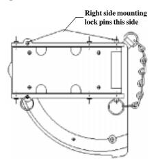
Assembly shown for left side of vehicle mounting. For right side mounting, move lock pins to opposite side. See lock pin removal.
