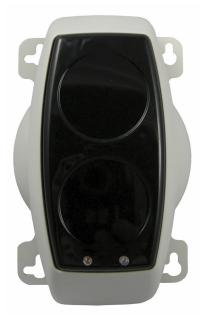
The Fyreye addressable reflective beam smoke detector comprises of a single unit incorporating an infrared transmitter and receiver. The signal is reflected by a prism and analysed for smoke presence. Should a predetermined level be reached, the detector will signal an alarm.
