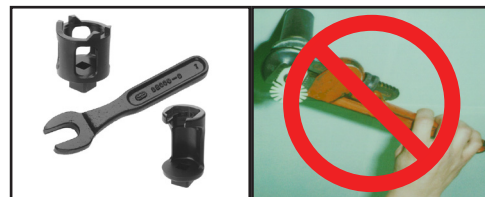
CORRECT (Special installation wrenches)
