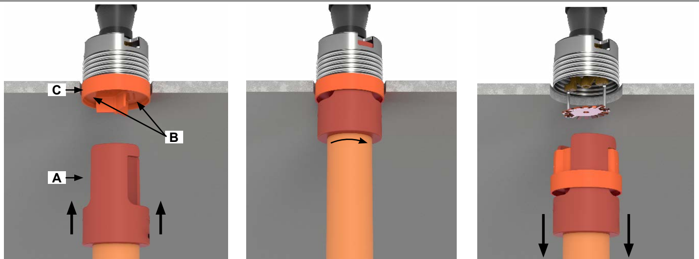
Figure 6: Using the Sprinkler Wrench
