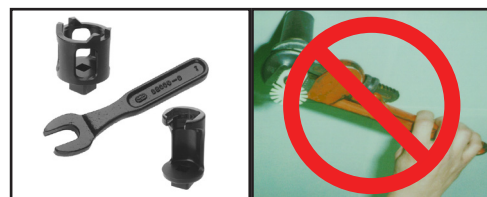
CORRECT (Special installation wrenches)
