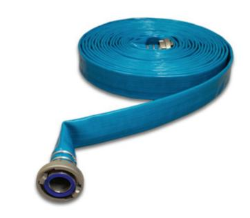
Circular woven jacket out of 100 % high tenacity polyester yarn with a thermoplastic Polyurethane liner and cover manufactured using the "Through-the-weave-extrusion-process."
