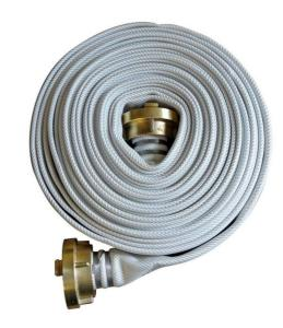
Standard firehose. High quality lay flat hose for all fire-fighting operations. Circular woven jacket out of 100% high tenacity synthetic yarn with an inner liner made out of a vulcanized high quality EPDMcompound.
