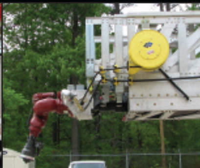
Single electric remote monitor and nozzle with controls at the tip and pump panel.
