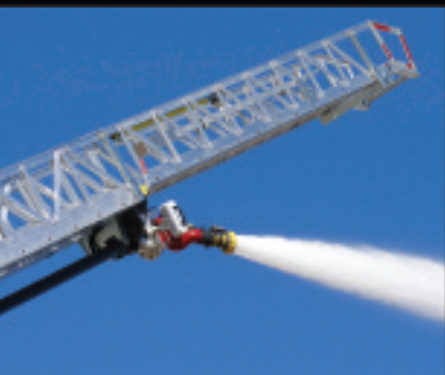
750 lb. tip load while flowing water and 1000 lb. rating when dry.
