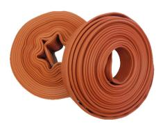
**Ozone Resistance:** When evaluated in accordance with standards ASTMD518, procedure B, 70 hours at 118°F, 100pphm of ozone, the cover or liner shows no visible signs of cracking.
