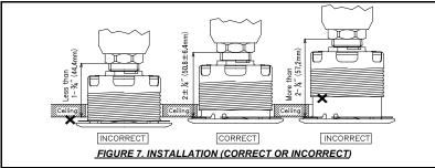
If the ceiling is to be repainted after the installation of the Sprinkler, care must be exercised to ensure that the new paint does not seal off any of the air gap. Factory painted Cover Plates must not be repainted. They should be replaced, if necessary, by factory painted cover plates. Non-factory applied paint may adversely delay or prevent sprinkler operation in case of a fire
