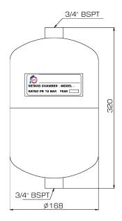
The RD Retarding Chamber is used with the Alarm Valve Trim when variable pressure is anticipated in the system. It is a holding tank to prevent the sounding of the sprinkler alarm during a water pressure surge, but will permit the sounding of the alarm on a sustained flow. The retarding chamber is connected to the alarm port of the alarm valve through the restriction nozzle. The retarding chamber is part of UL Listed Alarm Valve Trim. The retarding chamber is made of stainless steel material.
