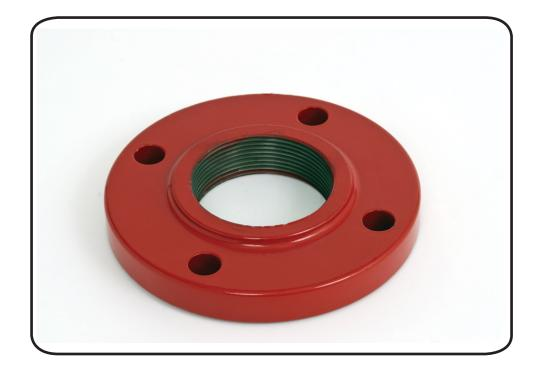
**Companion Flange** 2-1/2" (64mm), 3" (76mm) or 4" (102mm) with NPT female thread on the inside diameter to mount onto a male thread discharge pipe. Ideal for use with a butterfly valve between flange and monitor base. Red powder coat finish to match monitor.
