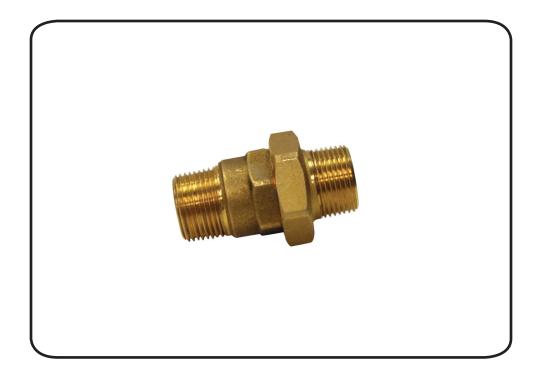
**Drain Outlet** is cast brass straight connection, male 3/4" NPT both ends. Used to drain low point of system between fire department connection and swing check valve. Seals automatically under pressure. Installed in horizontal position only.
