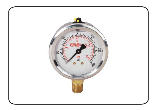
**Pressure Gauge** is stainless steel and liquid filled with a protective cover. 0-300# mounted on monitors at the base of the nozzle so that operator can insure proper pressure ranges for maximum, effective operation of both straight bore and combination fog/straight stream nozzles.
