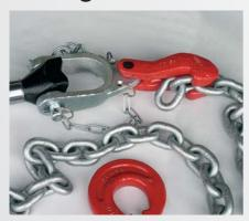
LANCIER Hydraulik pulling chains can be attached directly to the tips of the rescue rams LH-R-1800 and LH-R-11100 without tip exchange.
