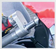
Base plates and wedge heads extend the operating ranges of LANCIER Hydraulik rescue rams.
