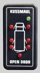
The Open Door Display provides a graphic representation of doors that are either open or ajar. One LED is wired to a switch at each compartment door. When the compartment door is opened, the switch provides an electrical path to ground to Illuminate an LED. Simple and easily installed. The display enhances safety and ensures that the operator will not drive away with an open door. Also available in 10 doors (091-178-10A).
