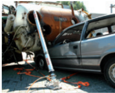
Heavy vehicle stabilization with hydraulic Locknut struts.
