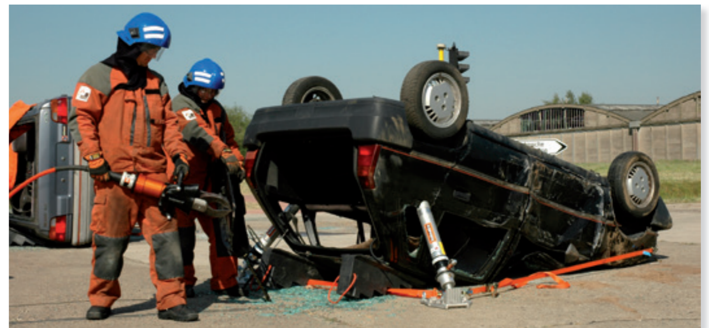
Two hydraulic struts used for light vehicle stabilization and, if required, controlled lifting.
