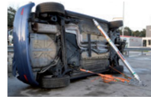
Extensions, heads and base plate used for light vehicle stabilization.
