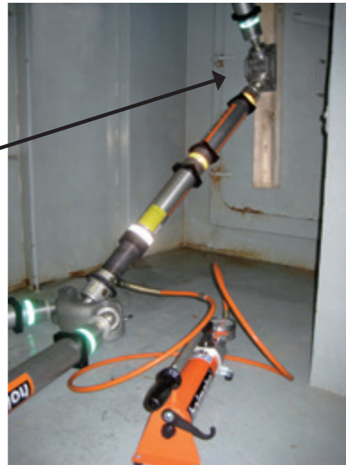
A 3-way swivel head and a 2-way block used for shoring lines in various directions.
