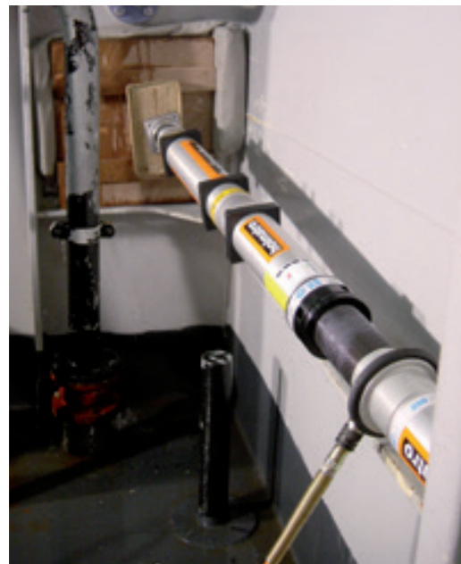
Sealing a leak in a dividing wall with the hydraulic PowerShore naval damage control system.
