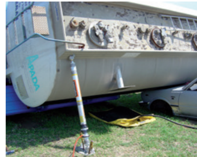
Pneumatic Auto-lock strut used for follow-up shoring in heavy vehicle lifting operations.
