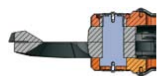
Squeezes blades directly for a superior cutting performance.
