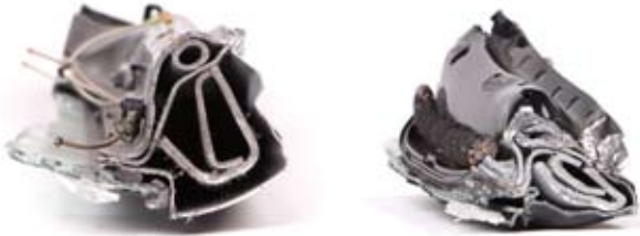
Cross section of the A-pillar of a new Saab 9-3 convertible before and after cutting.
