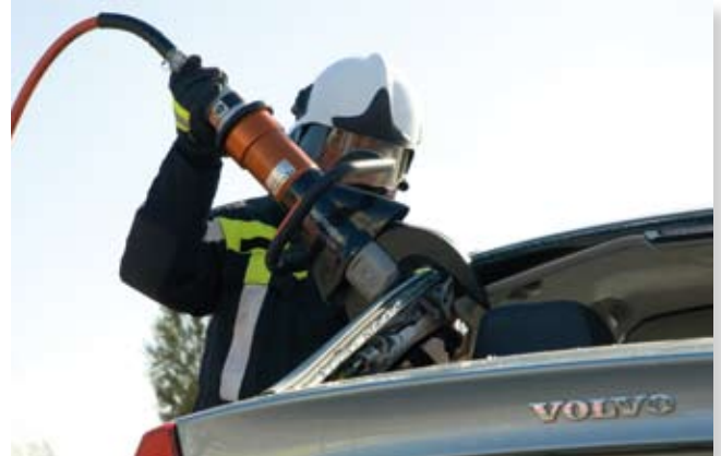
The CU 4055 C NCT™ II has been tested extensively on the wide A-, B- and C-pillars of the latest car models.
