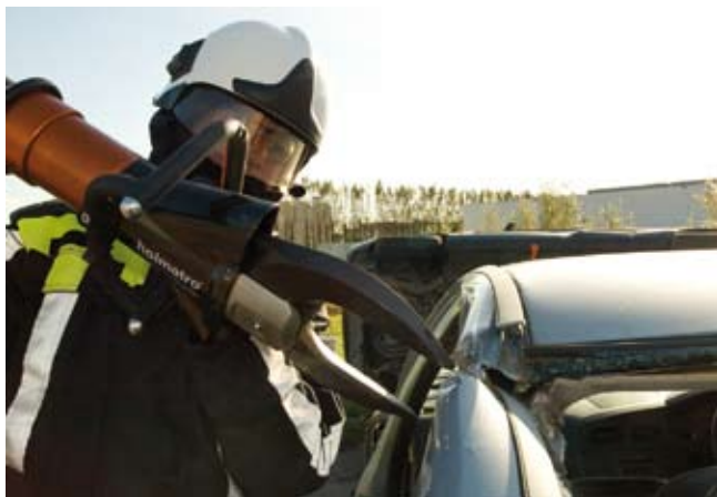
Wide Volvo C-pillar cut by CU 4055 C NCT™ II.
