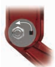
QUIK-ALIGN® — Rotating the eccentric collar allows up to 1 inch of axle alignment per side
