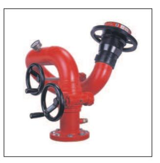
The monitor has welded stainless steel 4 inch (100 MM) waterway. The vertical and horizontal rotation is through bronze swivel joints with double row of stainless steel ball bearing. Both vertical and horizontal movements are controlled with handwheel driven enclosed worm gear.
