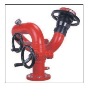
resistance. The vertical and horizontal rotation is through corrosion resistant bronze swiveling joint with double row of stainless steel ball bearing. Both vertical and horizontal movements are controlled with handwheel driven fully enclosed worm gears and protected from the elements.
