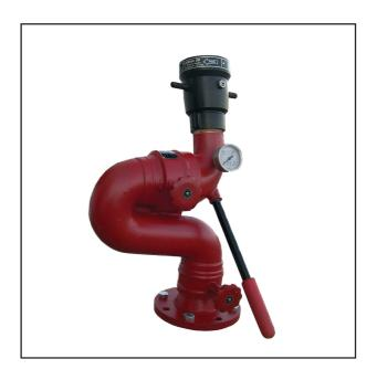
The monitor has cast bronze 3 inch (75 MM) water way. The vertical and horizontal rotation is through corrosion resistant bronze swiveling joint with double row of stainless steel ball bearing. Both vertical and horizontal movement are controlled by handle with twist lock.
