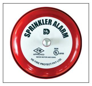
pipe must be used to reduce hydraulic friction loss. The Sprinkler Alarm should not be located more than 1.8 mtrs. (Six feet) above Alarm Valve / Deluge Valve. One Sprinkler Alarm may be connected to one or maximum of three alarm lines of seperate fire systems. For interconnecting more than one Sprinkler Alarm, a swing check valve in each line need to be provided.
