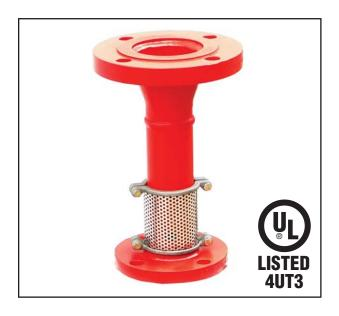
stream. The air is drawn into the foam solution through holes located on the foam maker covered with stainless steel screen to exclude nesting birds and insects. The aerated foam is directed into the pourer for the gentle application of the expanded foam. The pourers are available in different models.
