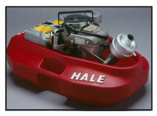
The Fyr Flote is a lightweight, portable centrifugal pump mounted on an unsinkable, high-strength polyethylene float with dual carrying handles and a splash suppression collar. A high-volume model (20FV-C8) and a high-pressure model (20FP-C8) meet most every pump need — in as little as four inches of water. Weighing just 49 pounds, the Fyr Flote stores easily in most truck compartments. It includes an automatic recoil starter, a spark arresting muffler, and an engine overspeed control switch.
