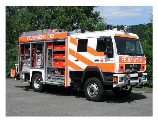
The TLF-OS on MAN 14.225 LA-LF acts mainly for the fire fighting, for delivering water, for handling simple technical rescue works and first-aid-measurements in the tunnel. With its crew it provides an automatic tactical unit. The crew of the TLF-OS consists of 1 + 4 persons. Furthermore the TLF-OS is equipped with a high-performance ONE SEVEN® 2100 E compressed air foam system in connection with the integrated centrifugal pump 16/8.
