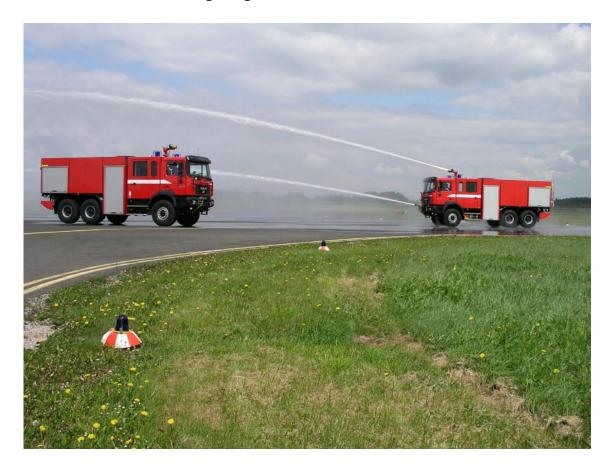
The TLF 60/80 had especially been built for the operation in China. The body of the vehicle consists of a light metal-box body where a 8,000 l water tank and 2,000 l foam concentrate tank for conventional foam concentrate, the ONE SEVEN® compressed air foam system "OS 3100 E" as well as a decontamination unit "deFcon 200" had been integrated.
