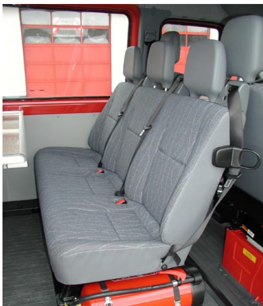
Additional bench, mounted contrary to the driving direction
