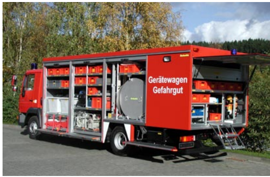
Deep-drawn shutter construction with retractable steps
