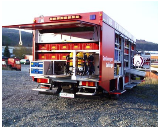
Vehicle rear with all storages for the personal equipment
