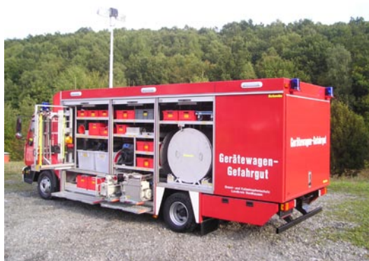
Left vehicle side - deep-drawn shutter
