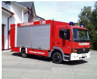
Shutter construction with rear cell
