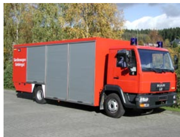
Deep-drawn shutter construction with rear cell
