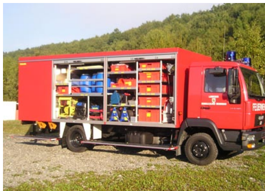
Shutter body with lateral protection foldable as step
