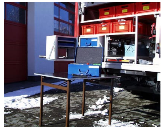
Free arrangeable working table with case for measuring devices
