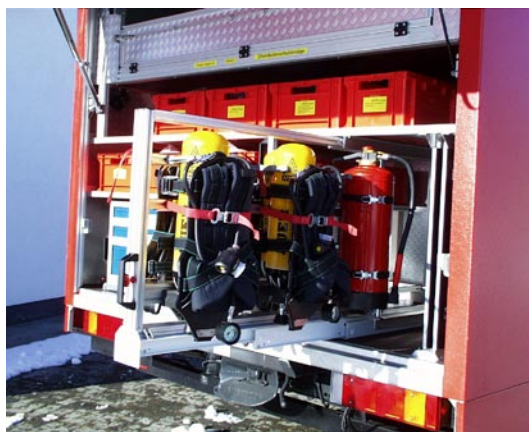
BA/spare bottle on extractable slide
