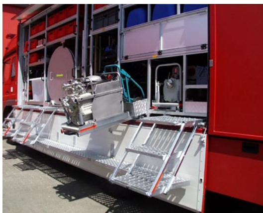
Steps for the upper equipment compartments and the hazmat persaltic pump on slide that can be lowered
