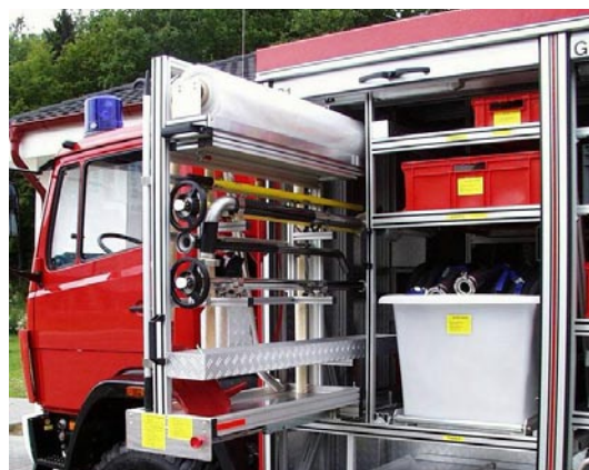
Sliding wall and storage 220l-PE-container
