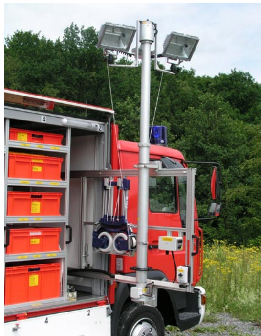
Lighting mast mounted in the inside
