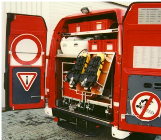
Rear equipment compartment with BA-storages
