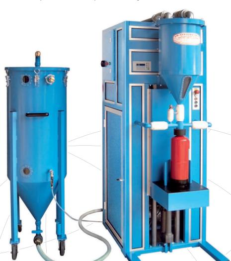
The unit operates within the filling tolerance indicated in the EN3 standards. Adjustment of the value of the filling weight has to be effected at the scale display; adjustment of the filling parameters depending on extinguisher type are effected by the text display. Height adjustment of the weighing platform takes place by screw-drive.
