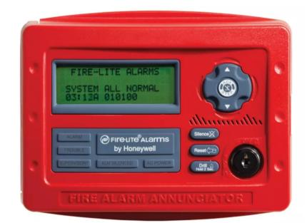
ANN-80 remote annunciators are compact, backlit, 80-character LCD fire annunciators that mimic the fire alarm control panel (FACP) display. They provide system status indicators for AC power, alarm, trouble, supervisory, and alarm silenced conditions. These annunciators communicate with the FACP over a 2-wire serial interface employing the ANN-Bus communication format. Connected devices are powered (via two additional wires) by either the host FACP or a remote UL Listed, filtered power supply.
