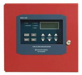
The ANN-100 annunciator provides system status indicators for AC Power, Alarm, Trouble, Supervisory, and Alarm Silenced conditions. The ANN-100 and the FACP communicate over a two-wire serial interface employing the ANN-BUS communication format. Connected devices are powered via two additional wires, by either the host FACP or a remote UL-listed, filtered power supply.
