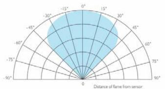
To meet the requirements of EN54-10:2002 clause 5.4 (Directional Dependence), viewing angles must not exceed ±30°.
