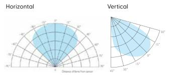
To meet the requirements of EN54-10:2002 clause 5.4 (Directional Dependence), viewing angles must not exceed  $\pm 20^{\circ}$ .
