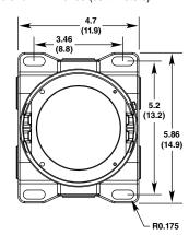
Class I, Div. 1, Groups B, C & D (T5); Class I, Div. 2, Groups B, C & D (T4); Class I, Zone 1/2 AEx d IIC (T5); Class II/III, Div. 1/2, Groups E, F & G. Tamb -40°C to +75°C NEMA/Type 4X, IP66 Conduit seal not required. Performance verified in accordance with:
