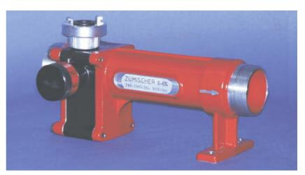
The Z - 800 in-line inductor is constructed for a pre-calculated water flow. It creates a pressure drop in the water pressure of only about 30-33% at that flow. Foam is drawn through a 25 mm pickup tube from a container at atmospheric pressure. The flow of foam concentrate is continuously added to the water stream.
