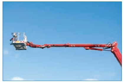
Extended up-and-over capability up to 11 meters - improved manoeuvrability in congested areas.
