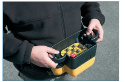
Radio remote control for all boom movements and other fire-fighting functions.
