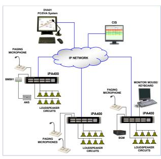
The iPA400 can be controlled from an ASL or third party workstation in the IP network, or can have a directly connected monitor, mouse and keyboard, or touchscreen.
